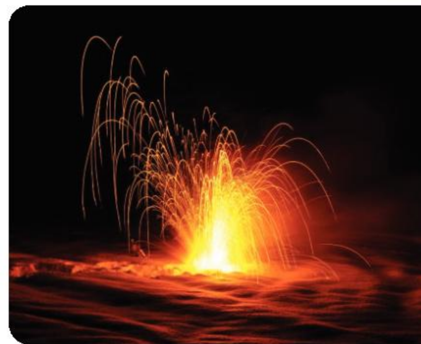
▲ Sodium and potassium react vigorously with water, releasing hydrogen gas that can ignite
